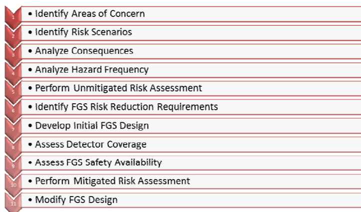
Figure 1 – Fire and Gas System Lifecycle ISA TR 84.00.07
