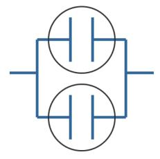
Two-out-of-two voting (2002) also employs two devices. In this arrangement, of the two devices, both devices must "agree" to cause a shutdown before the shutdown will occur. I.e., both devices must vote to trip to cause a trip action. This is physically represented by two switches in parallel. De-energizing either the "A" switch or the "B" switch alone will not cause the entire circuit to de-energize. Only when
